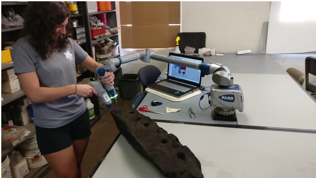
Here, M.S. student Julia Herbst scans a timber using the FARO arm.
