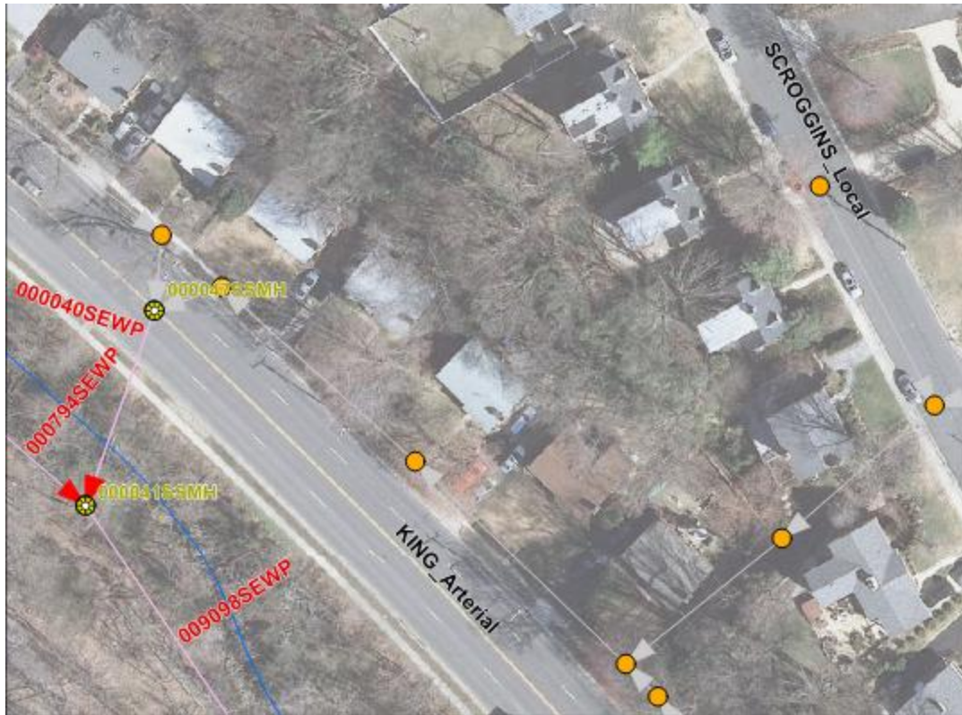
Figure 4-7: Location of exposed side sewer crossing 000040SEWP along Taylor Run
