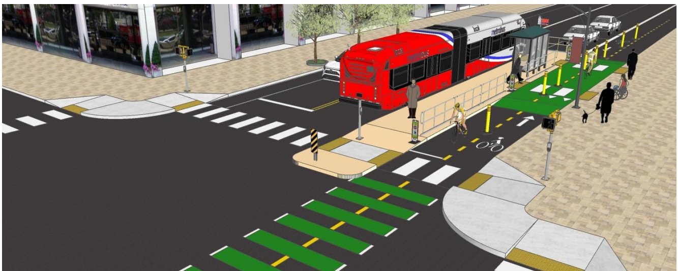
Figure 29: Boarding Island Bus Stop with Pedestrian Refuge Island in Crosswalk
