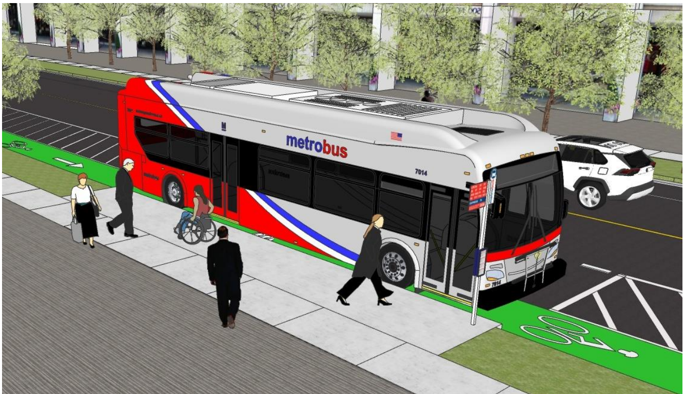
Figure 41: Mixing Bike/Bus Stop
