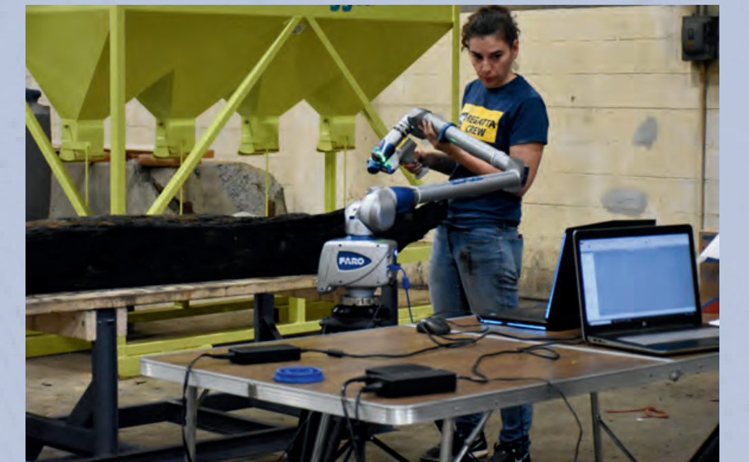
Laser scanning ship timbers
