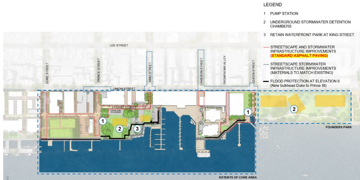
Figure 1: Proposed Phase 1 Waterfront Flood Mitigation Improvements
