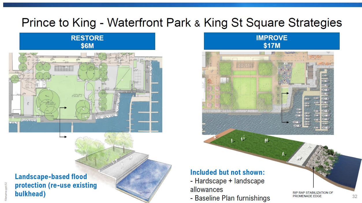
Figure 3: Landscape-Based Flood Protection at Waterfront Park
