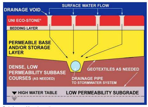
Typical permeable paving section
