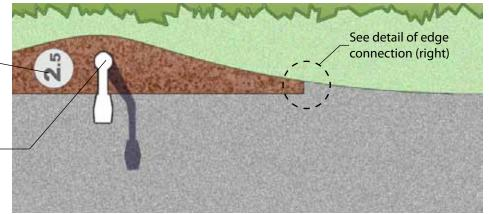
The edge connection of the asphalt path is designed to eliminate a narrow area which would be difficult to construct
