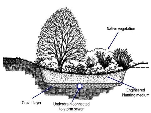
Typical bioretention detail
