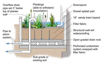
Typical stormwater planter installation detail
