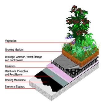
Typical green roof installation detail, depth of growing medium varies greatly from a few inches to several feet, depending on roof structure and desired planting types.
