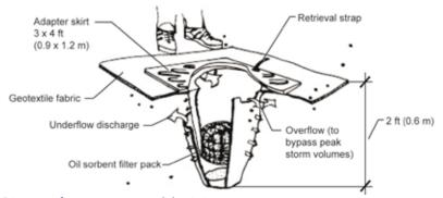
Diagram of a stormwater catch basin insert
