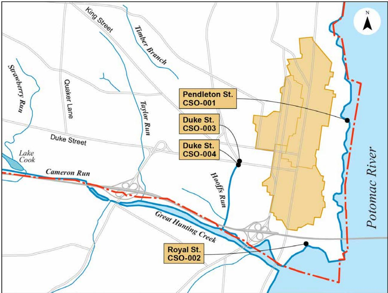
FIGURE 3-1. COMBINED SEWER OUTFALLS IN THE CITY
