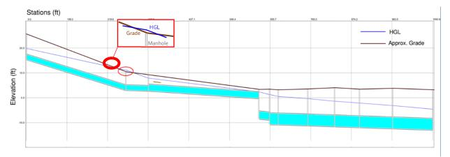
Figure 1 Example of a Storm Sewer Street Flooding Location in XPSWMM
