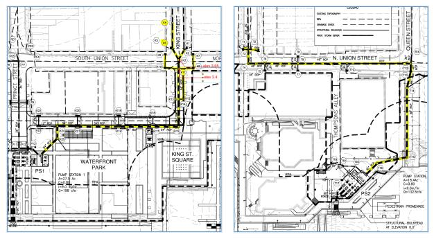
Figure 7 PS1 Storm Sewer (Left) and PS2 Storm Sewer (Right) Revised Depths
