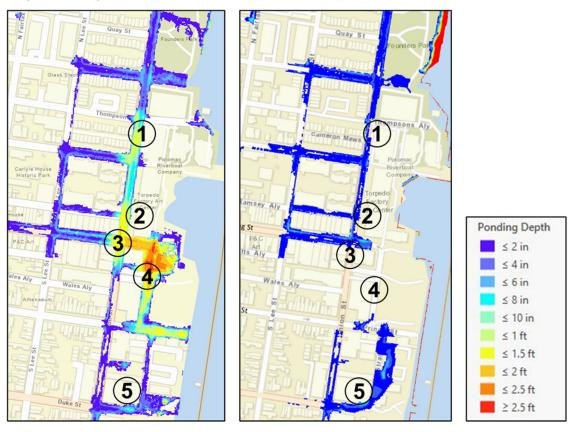
Figure 3 Design Storm Projected Street Flooding for Existing Conditions (Left) and Baseline Project (Right)
