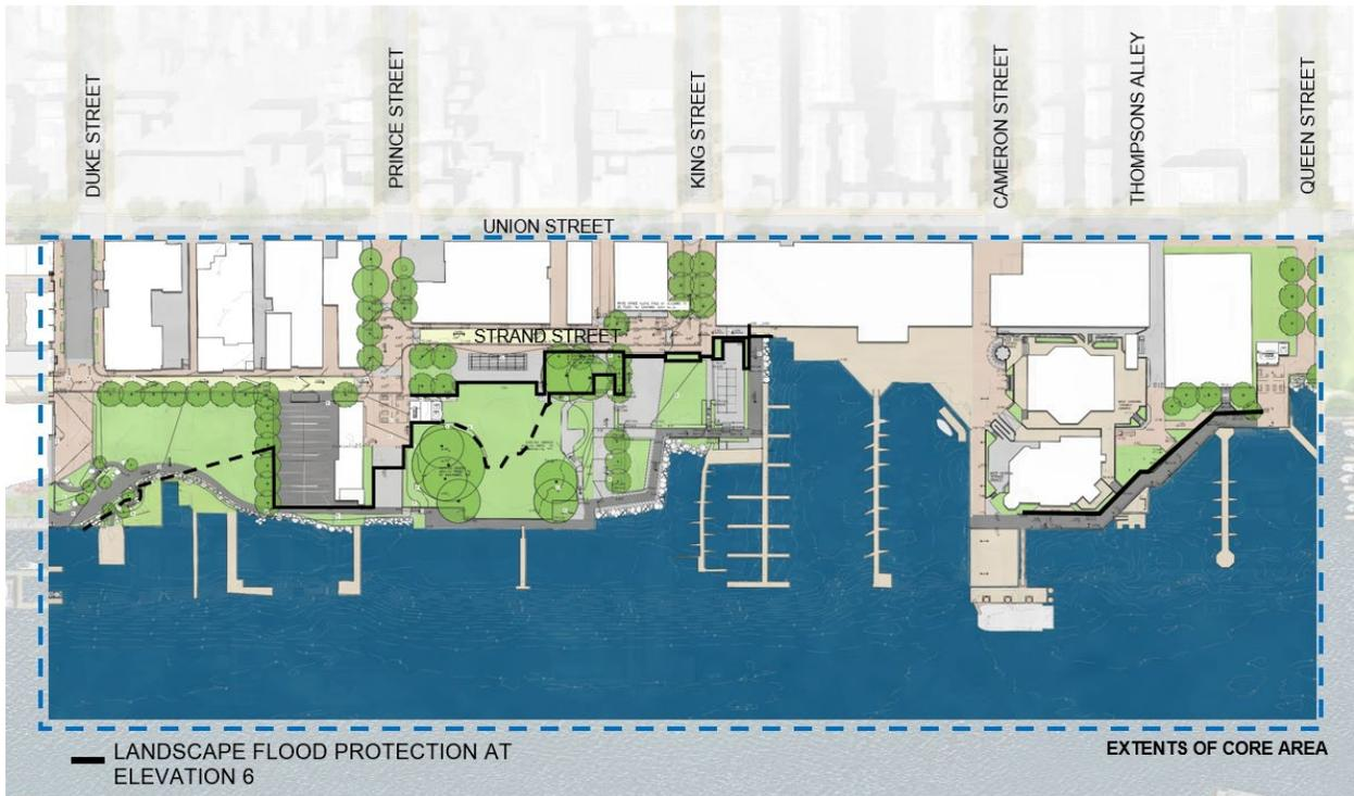
Figure 13 Landscape Flood Protection at the Strand and Maintaining Shoreline Alignment
