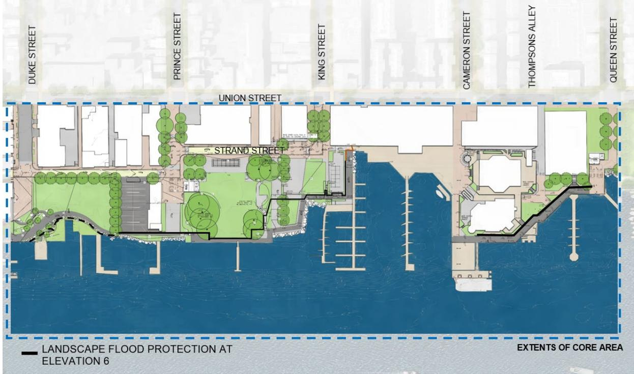
Figure 12 Landscape Flood Protection at the Waterfront and Maintaining Shoreline Alignment
