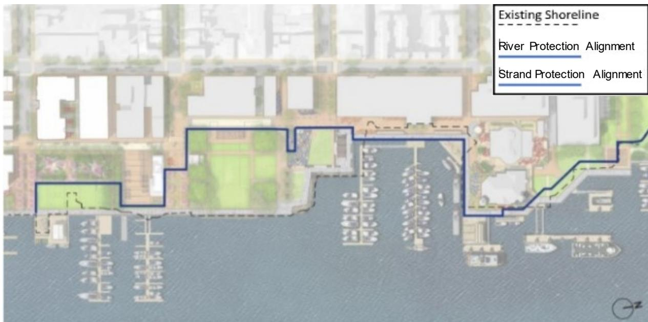
Figure 11 Value Engineering Solutions Providing El. +6.0 ft Flood Protection at the River and at the Strand with Landscape-Based Flood Barriers
