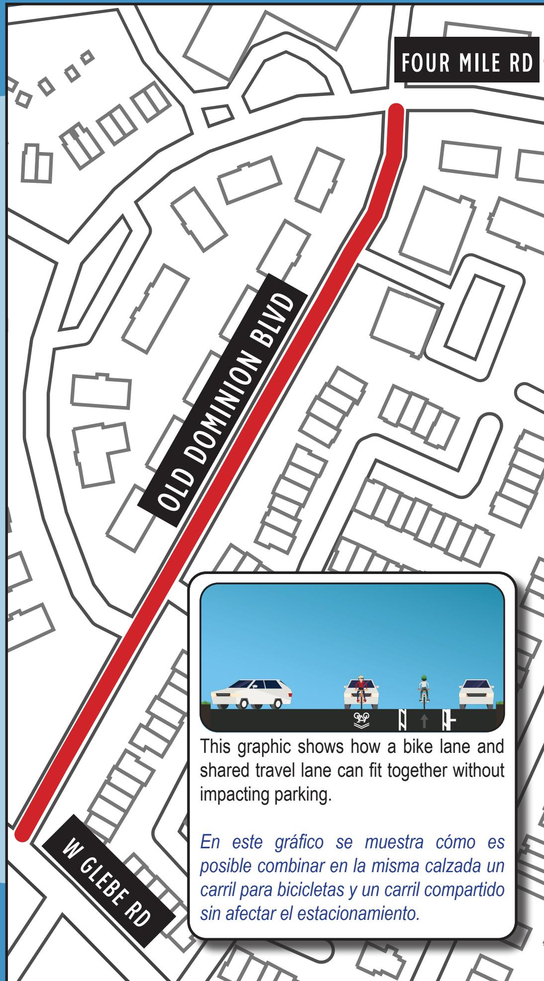
This graphic shows how a bike lane and shared travel lane can fit together without impacting parking.
