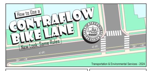
Contraflow bike lanes allow bicyclists to move in two directions on one-way streets, providing convenient and direct connections between bike routes.
