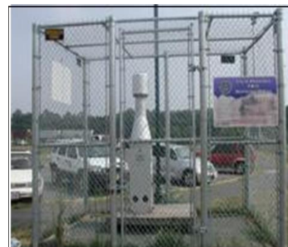
PM 10 air monitoring station at Cameron Station
