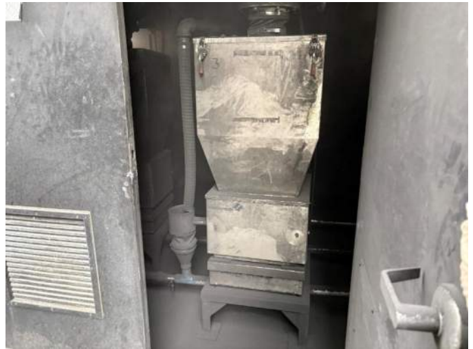
Figure 6: Carbon silo appears to have minimal emissions
