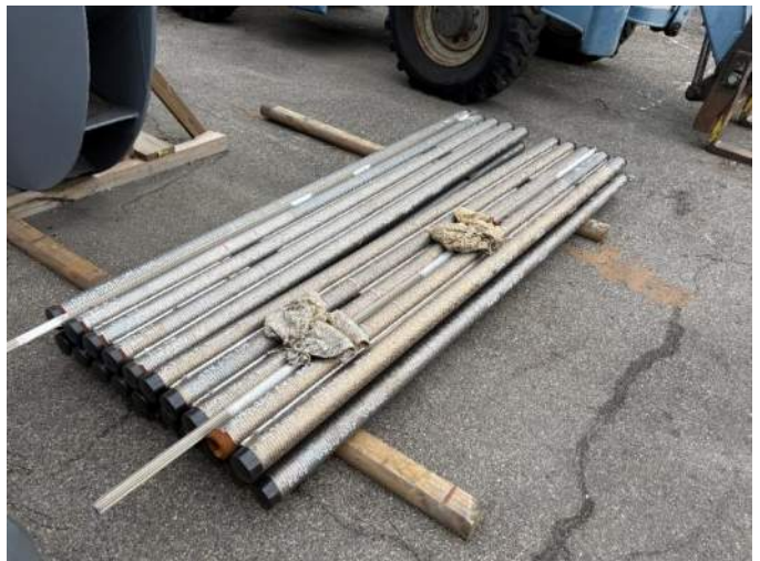
Figure 10: Unit 3 spiral wound Inconel waterwall tube pendants
