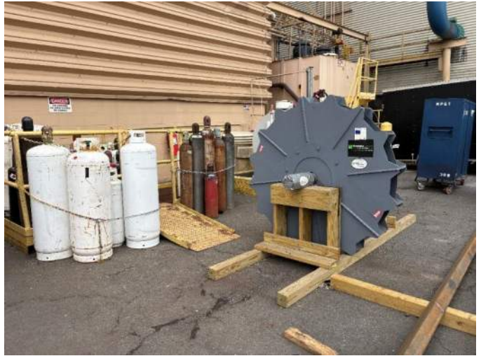
Figure 8: Spare rotor for under fire air fan
