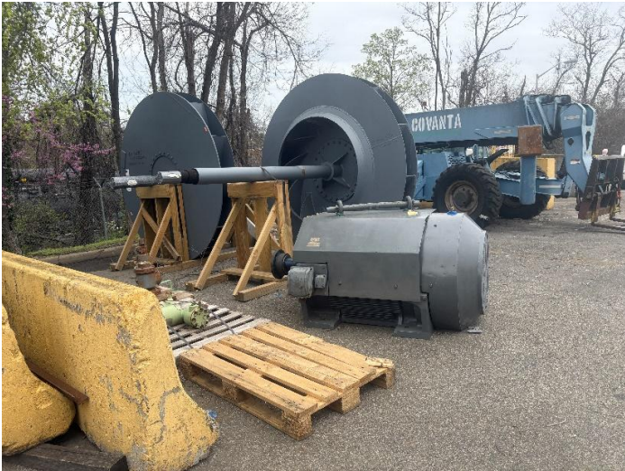
Figure 7: New Induced Draft Fan Rotors Being Stored
