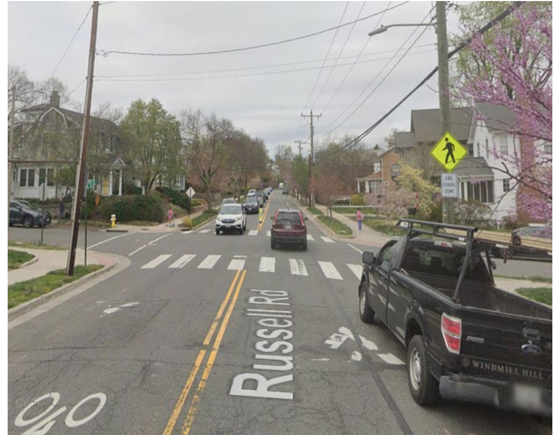
Parked vehicle blocks sight of curb ramp
