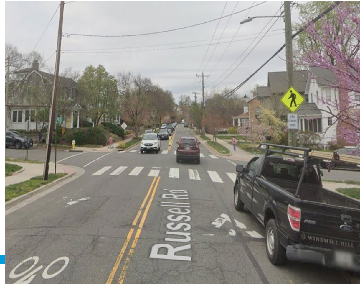
Parked vehicle blocks sight of curb ramp
