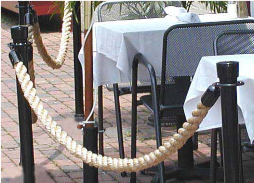
FIGURE 3 Rope or chain barrier must have a minimum diameter of 1 inch
