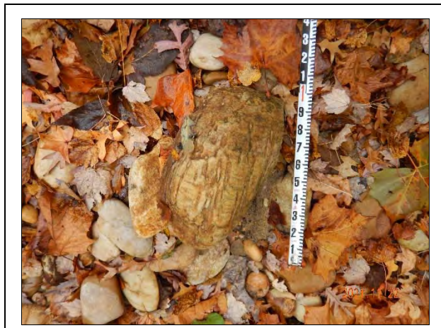
Figure 41. Typical Largest Particle (305 mm) Observed Along the Streambed
