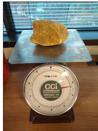
Figure 42. Weighing Largest Point Bar Sample Particle (105 mm)
